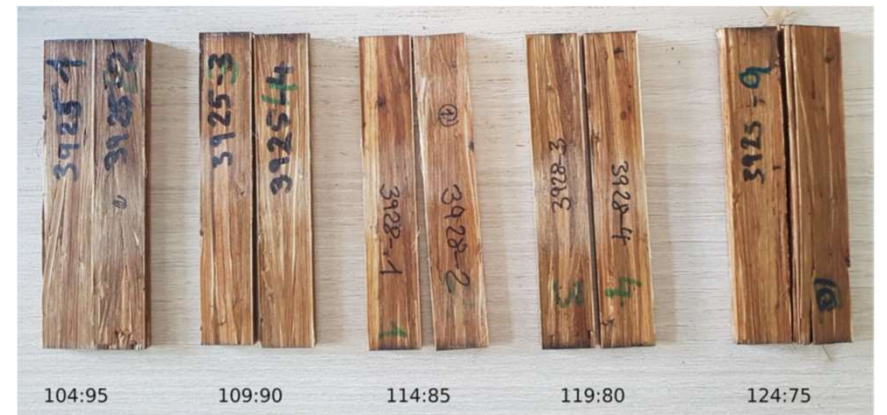
Trials with different ratios of synthetic raisin and chemical hardeners (© K. Dippon, B.A.M. GmbH)
