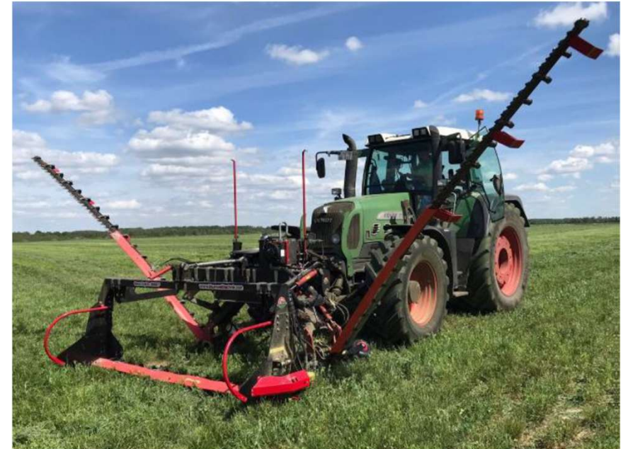
Adapted mower for high-cut harvesting (© J.Bachinger, ZALF)
